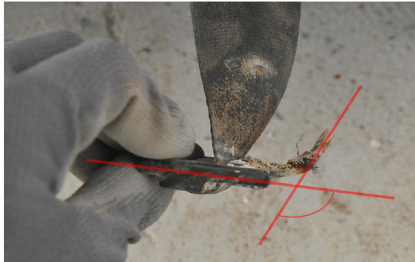
Figure 84: Malformation of the crotch belt fastening
