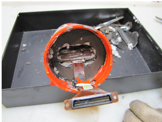
Figure 22: CVR memory board after removal of thermal protections
