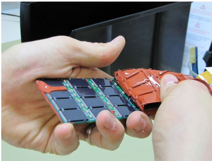
Figure 20: Removal of internal protective layers
