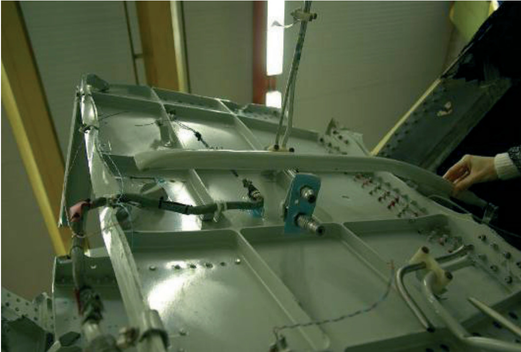
Deformations of the rudder control rod consistent with the backwards indentation of frame 84
