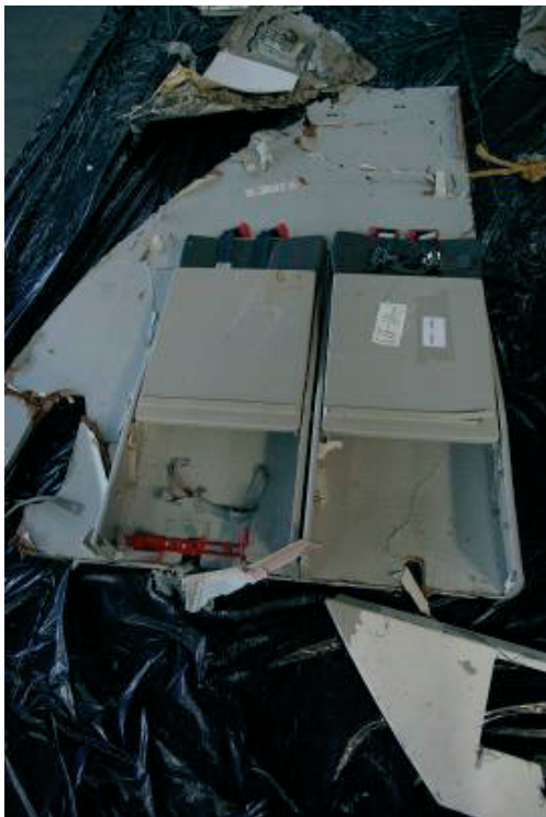
Cabin crew seats located on the toilet L11 partition at the level of left-hand door 1
