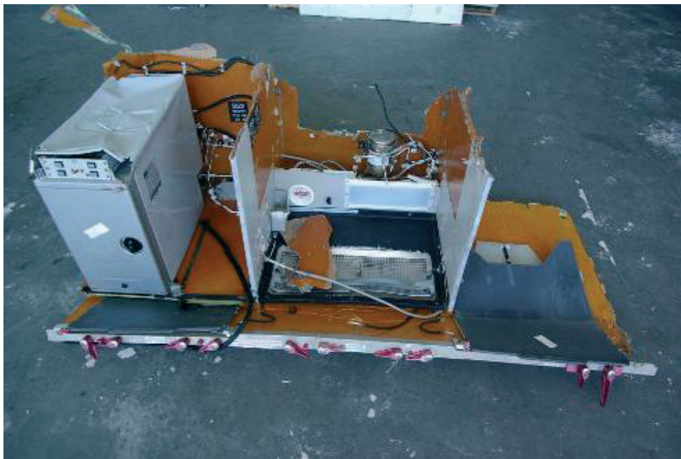
Part of Galley G3: downwards deformation at the level of the galley's heavy parts
