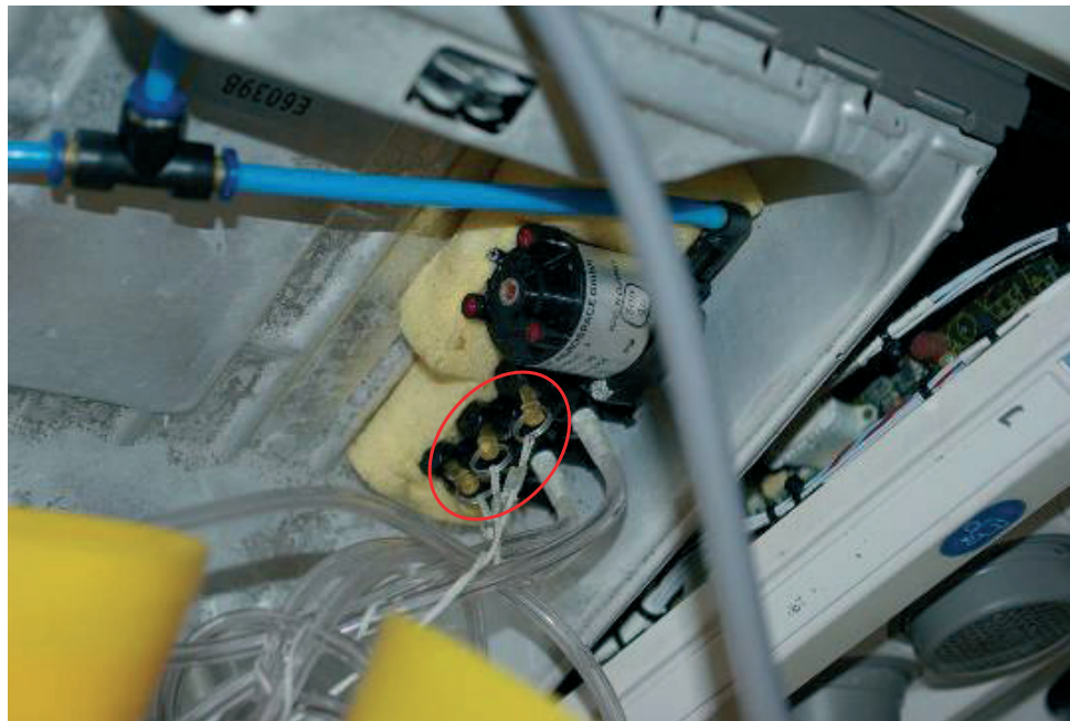
Passenger oxygen container recovered open: the three pins are in place
