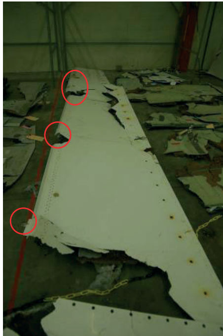
Outboard half of the right-hand elevator: the four attachments that can be seen were deformed bottom-upwards
