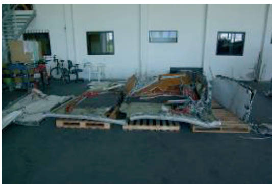
Floor of the LDMCR: with bottom-upwards deformation
